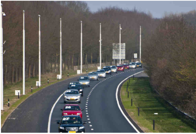
Figure 2. Overview of the test site, in use for the closed track experiments of the SPITS project. A fixed camera of the VBM system is installed on every pole, which are positioned 100m apart.
